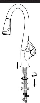
Remove the rubber, metal washers and mounting nut from the base by hand twisting it off.
