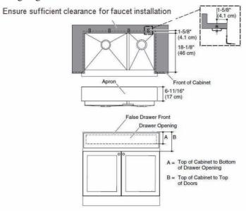
IMPORTANT! Before installing this sink, verify the opening height (A) is less than the apron height and the distance to the top of the doors (B) is greater than the apron height.
