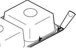
□ Apply a bead of silicone sealant to the edge of the sink.
