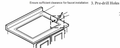
□ Ensure sufficient clearance for faucet installation, position with provided template on countertop. Locate the template front to rear, so that sink will not interfere with the cabinet. □ Trace a line around the template. Cut along the inside of this line to provide opening.
