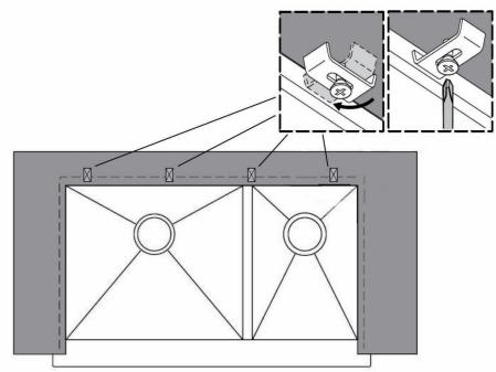
Determine placement of clip brackets. Pre-drill holes according to method desired D Position and align sink over opening. Press sink onto Silicon seal. After re-checking alignment, install the clips to the countertop, ensure each clip engages the rim. Tighten evenly. □ Remove excess sealant and dry for at least 24 hours.
