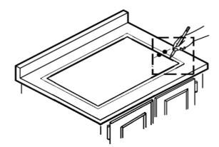
□ Use the provided cutout sheet to carefully measure and cut the countertop for the top-mounted sink. □ Please ensure all measurements are accurate and precise before cutting or drilling.
