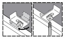
□ After re-checking alignment, install the clips to the countertop, ensure each clip engages the rim. Tighten evenly.
