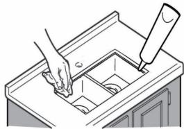
□ Remove excess sealant and dry for at least 24 hours.
