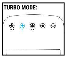
Press + to start TURBO MODE for maximum fan power and cooling.
