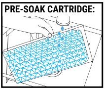
To **ACTIVATE COOLING**, soak your cartridge under running cold water.
