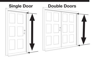
Standard security door handle height is 39-1/2". To check for potential interference with your main entry door handle, measure from the threshold to the center of the handle (Y). A measurement within 38-1/2"-40-1/2" inches may result in interference. To ensure you avoid interference issues in this instance, you may:
