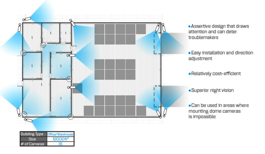
**Bullet camera** is a favorite for most surveillance system installers simply because it is the easiest one to install. There is no need to take anything apart – one simply mounts the base on the wall or ceiling and screws it in place. The actual camera can then be swiveled up and down depending on the area of view you want to cover. Due to ease of installation and adjustment, bullet cameras are popular for outdoor use.
