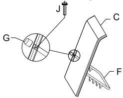
Put plastic cap (G) on option frame, then connect the frame with backrest (C). M6\*40 bolts (J) are used. Please tighten bolts to the end.
