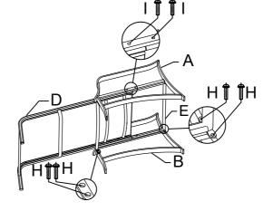
Connect armrests (A and B) with seat board (D) and across beam (E). M6\*15 bolts (H) are used. Please do not tighten bolts to the end at this step.
