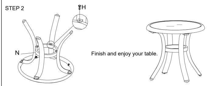
Connect table leg support ring (L) with table legs. M6\*15 bolts (H) are used. Make sure all bolts are connected properly, then tighten all bolts to the end.
