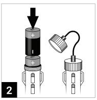
Add four new D size batteries to the battery pack
