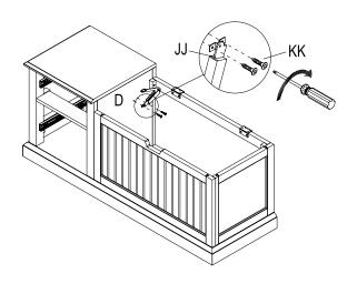
$\hfill \Box$  b) Attach panel (B) to assembled body with screw (KK) as shown.
