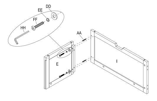
b) Attach panel (E) with washer (DD), spring washer (EE), and bolt (FF).
