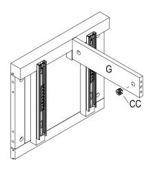
□ c) Join bar (G) to the panel (D) with dowel (AA).
