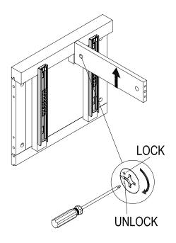
Wood dowel Cam lock bolt Cam lock Small head Large head
