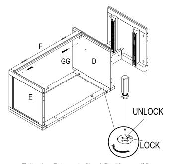
e) Tighten bar (F) to panels (D) and (E) with screw (GG).
