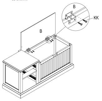
c) Attach safety hinge (JJ) to panel (B) with screw (KK) as shown.
