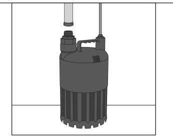
1. Select the correct adapter attachment for connecting the discharge line dependent on the pump application
