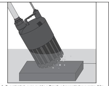
5. To avoid airlock, pump must be sufficiently submerged before pumping. If the pump is not pumping, tilt the pump to release the air bubbles from the bottom, then return to the vertical position. Unplug the pump from its power source when finished pumping, do not let the pump run dry.
