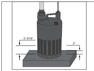
Install the pump on a firm, level base. Avoid pumping mud, rock, or other debris.
