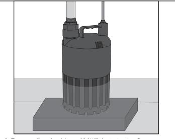
3. The pump will need a minimum of 2-9/16" of water to prime. Once primed, the pump can remove water down to 2"
