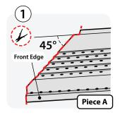
Cut the end of Piece A at 45-degrees. Next, cut a 1/2 inch wide notch from the back wing. Then, trim off 3/4 to 1 inch from the front edge in a straight line.
