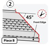
Cut the end of adjoining Piece B at 45-degrees. Repeat the 1/2 inch wide notch cut on the back wing and the 3/4 to 1 inch trim from the front edge. Pieces A & B should slightly overlap.
