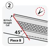
Cut the end of Piece B at 45 degrees. Next, notch the edge of the back wing in a 1/2 inch straight line. Place Piece B atop Piece A and check that the alignment has no gapping.
