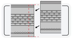
Slightly overlap the next guard so the perforated holes align with the previous piece. Follow the same screw pattern as the previous piece.
