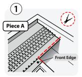
Trim the front edge of Piece A as shown in Image 1. Use the drain holes in the trough as a cut line. This will allow Piece B to fit properly atop Piece A.
