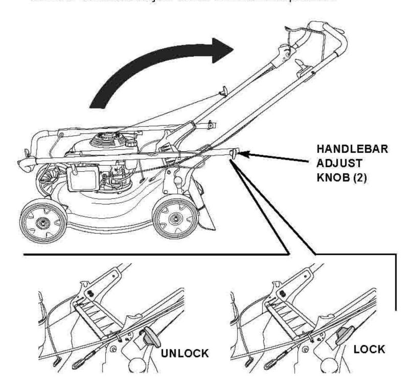
Turn the adjust knobs 90 degrees into the lock position so the pins will spring into the holes and lock into position.
