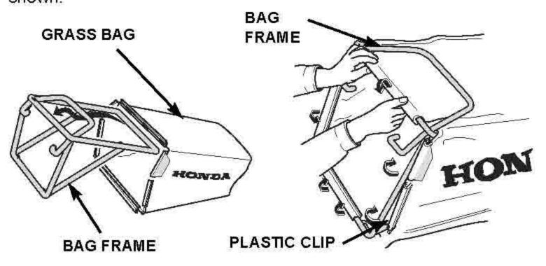
Lift the discharge guard, remove the mulching plug, and install the grass bag.
