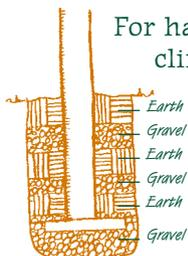
For harder, rockier soils and in colder climates, pour a bed of gravel into the hole, place a block of treated wood on the bed, insert the post, level it, and fill the hole with layers of earth and gravel, tamping frequently and leaving a mound at the top for drainage.
