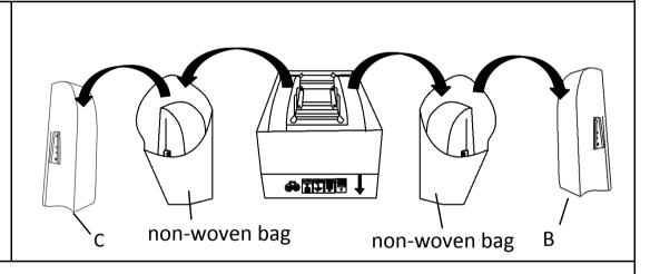
Take out 2 non-woven bags with Left Wing(B) and Right Wing(C) inside from the bottom of the armrest. Then take out the Wings from the non-woven bags.
