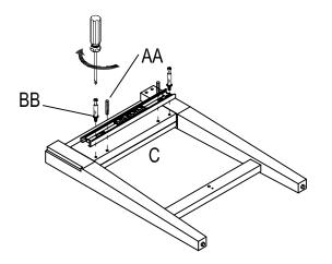
**c)** Join panel (D) to the frame (C) with dowel (AA).
