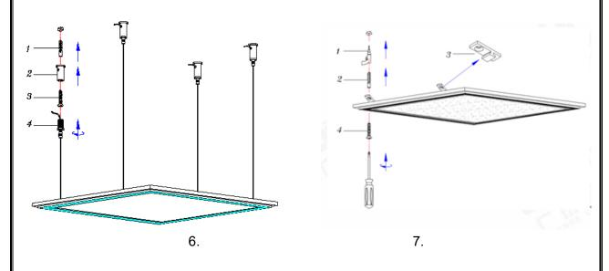
1. Make sure that the ceiling can hold the weight of the LED panel and install ceiling brackets
