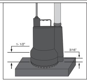
2. Install the pump on a firm, level base. Avoid pumping mud, rock, or other debris.
