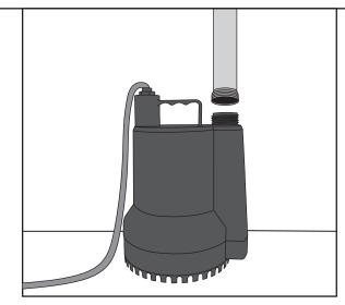
Attach 1" garden hose to the discharge of the pump. If a smaller 3/4" hose is preferred, attach the threaded adapter to the pump discharge before attaching the hose.
