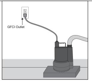
4. Plug the pump in to a 115V GFCI Power Outlet
