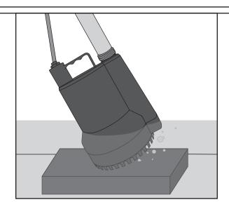
5. To avoid airlock, pump must be sufficiently submerged before pumping. If the pump is not pumping, tilt the pump to release the air bubbles from the bottom, then return to the vertical position. Unplug the pump from its power source when finished pumping, do not let the pump run dry.
