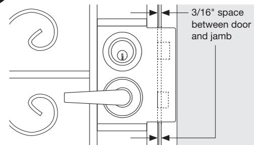
With the lock bolts extended, align the lock bolts with the holes in the lock-side jamb (B). Allow approximately 3/16" space between the door and the jamb. Make certain the jamb is plumb, and the top is level to the top of the hinge-side jamb.
