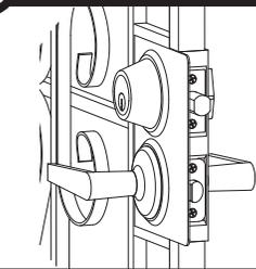
Install your choice of locksets with 2-3/8" backset (sold separately). Fully extend the lock bolts into the "locked" position.
