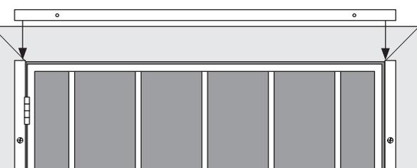
Position the top header jamb (C) across the top of the two side jambs. Make certain there is a minimum 1/8" space between the header and the top of the door frame, and that the header is level.
