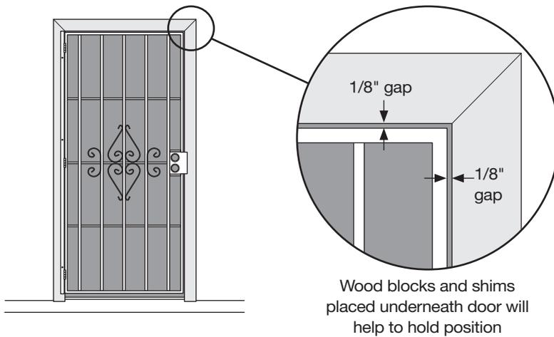
Wood blocks and shims placed underneath door will help to hold position
