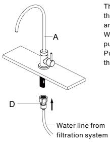
Thread the quick connect adaptor (E) onto the end of the faucet assembly (A) stud, and tighten securely using a wrench.
