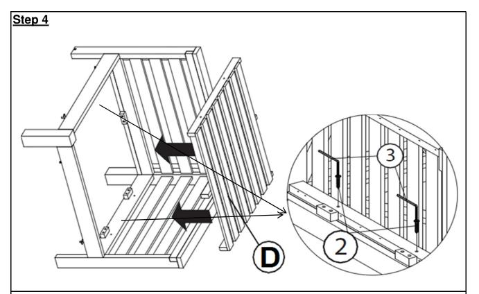
Attach the Seat Panel (D) into the Corner Chair as shown in picture above. Affix Seat Panel (D) with Corner Chair by using Screws ((2)) and Allen Key ((3)).
