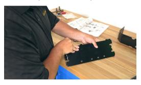
b. Flip over the assembly and mount the hitch support bracket, use the holes furthest away from the rear hooks and use two carriage bolts and the wing knobs to secure them
