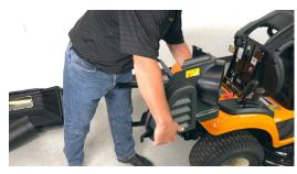
b. Slide the left side into the upper chute support using the tabs
