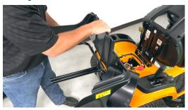
c. Align the cover tabs with the chute support, slide hinge pin in place
