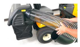
c. Slide the chute into the opening, turn counterclockwise until secure
