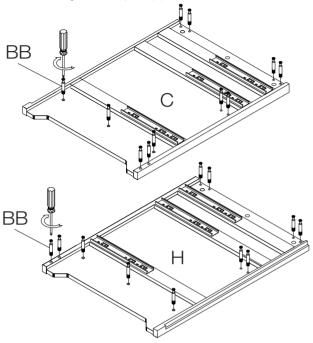
d) Connect right side panel(C) /middle right vertical panel(H) /front right horizontal panel (J) /Back horizontal panel(K) /right bottom panel(E) / Front bottom panel(F) with big Cam lock (AA)
