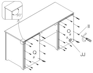
Big cam lock Big cam lock bolt Round head screw
