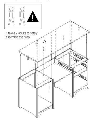
□ c) Connect the top panel with the big cam lock(AA)
