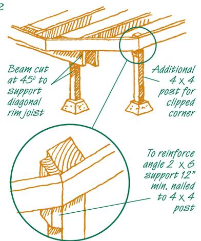
You may clip from 2' - 4' of the deck width or length, as long as in doing so, you do not eliminate a post. Remember, also, that by clipping the corner, you are removing some of the beam; therefore, you will need to install an extra post for support.
