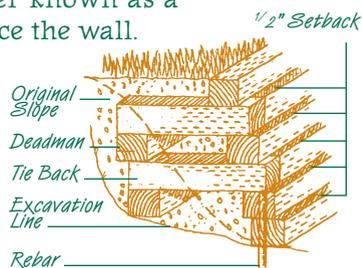
placement of the tie back and "deadman" will require more extensive excavation into the slope. These supporting timbers are leveled to lie on one course of wall timbers and are spiked into the timber below before setting the next course.
