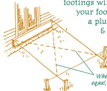
When diagonal lengths are equal, the footing positions will be square.
