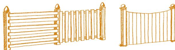
*Board on Board — Horizontal and Vertical    Curved Panel Picket*
