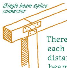
Therefore, make a second mark on each post below the first mark at a distance equal to the height of the beam. Then cut the posts at the second mark. Set the beam on top of the posts and attach with connectors and nails. Single beams are more susceptible to swaying, so use bracing wherever possible.
