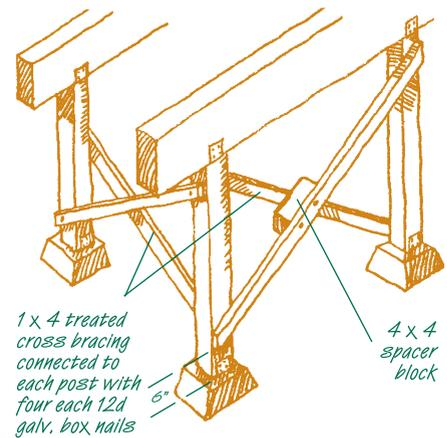
bracing requirements in your area. Refer to the illustration below when constructing your cross bracing.
