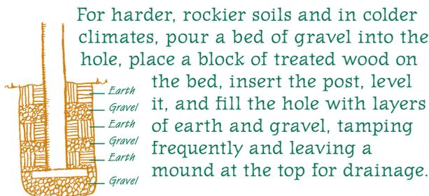
For harder, rockier soils and in colder climates, pour a bed of gravel into the hole, place a block of treated wood on the bed, insert the post, level it, and fill the hole with layers of earth and gravel, tamping frequently and leaving a mound at the top for drainage.
