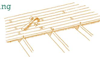
Secure the decking boards at each place where they cross a joist, using two nails or screws for 2x4's and three nails or screws for 2x6's. When using boards shorter than the deck length, make sure all board ends rest on a joist, and use different board lengths in order to stagger the splices.
