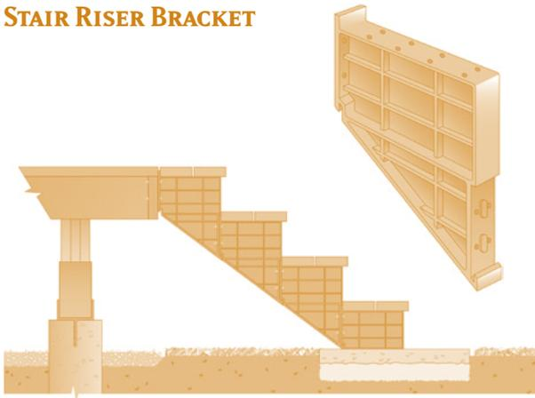
Stair Riser Brackets work in tandem to give strength and support while providing uniformity to your stair design. Easily bolted together, Stair Riser Brackets offer limited measuring to achieve maximum results.
