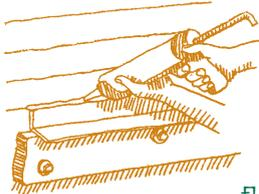
the house. Drill two holes at each midpoint between joist hanger marks, then permanently secure the ledger board to the rim joist with lag bolts. Add flashing and caulk.
