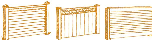
*Horizontal Louver (May also be vertical)    Lattice Top    Closed Post and Board*
