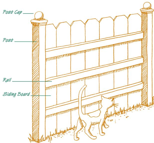
The components of most wooden fences include posts, rails, siding boards and post caps.
