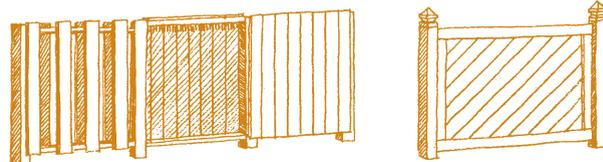
*Alternating Boards and Alternating Panels    Diagonal Board*
