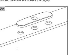
Install with Deck Plate. Place a bead of plumber's putty between faucet and sink. Place Deck Plate over the three holes of sink.
