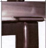
Step 3. Extend each Latch Plate up and over the lip edge and firmly tighten each T Knob. Brake should now be secured to Stand. Check T Knobs often and tighten as needed.
