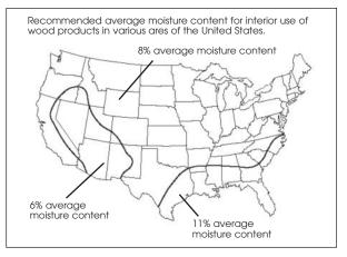
When installing Pergo flooring the maximum acceptable moisture reading for wood subfloors is 14%.
