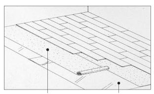
Pergo SilentStep™ Foam or Soundbloc™ Foam to be used with flooring that doesn't have attached underlayment.
