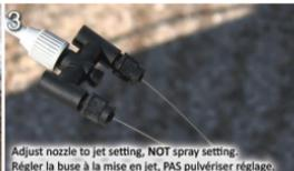
3 Adjust nozzle to jet setting, NOT spray setting.
