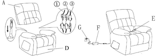
• STEP 6: Connect Transformer (F) with Motor (Assembled under the seat).
