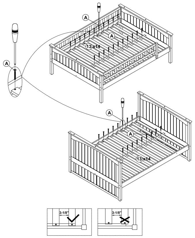
Note: Do not lock the screws of the bed slats to the outermost edge of the bed slats, you need to leave a certain space at the edges, otherwise it will cause the board to break
