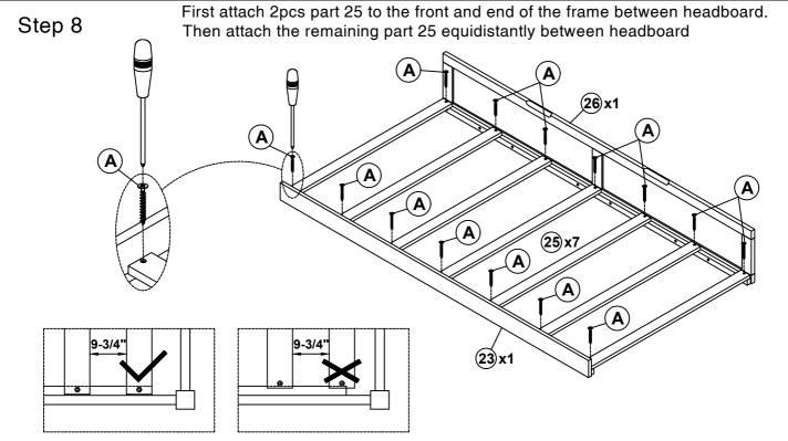
Note: Do not lock the screws of the bed slats to the outermost edge of the bed slats, you need to leave a certain space at the edges, otherwise it will cause the board to break
