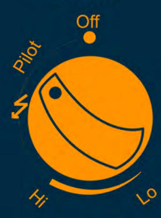
Push control knob and roatate counterclockwise until it stops at the pilot position.
