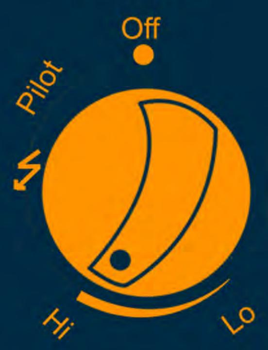
Push in and turn the control knob to the "HIGH", then release control knob.
