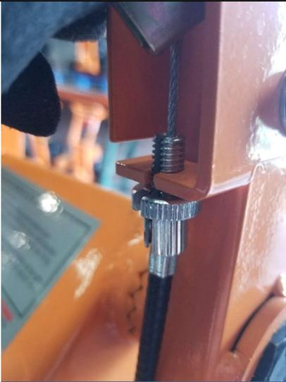
Adjust barrel adjuster to be able to slide in the brake cable.
