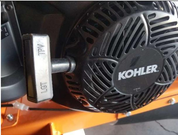
Engine recoil starter. Used to pull start the engine.
