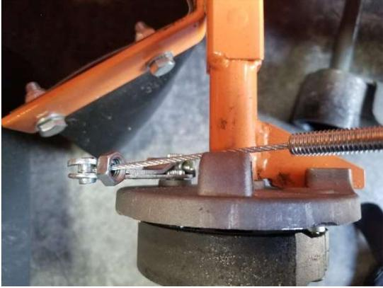
Loosen lock nut and install brake wire and brake adjuster into brake adjuster mount.
