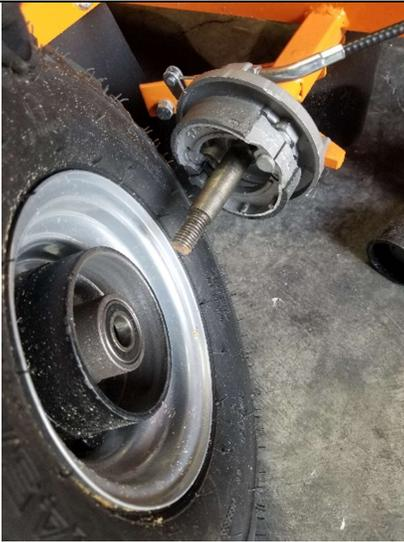
Install wheel with brake drum.
