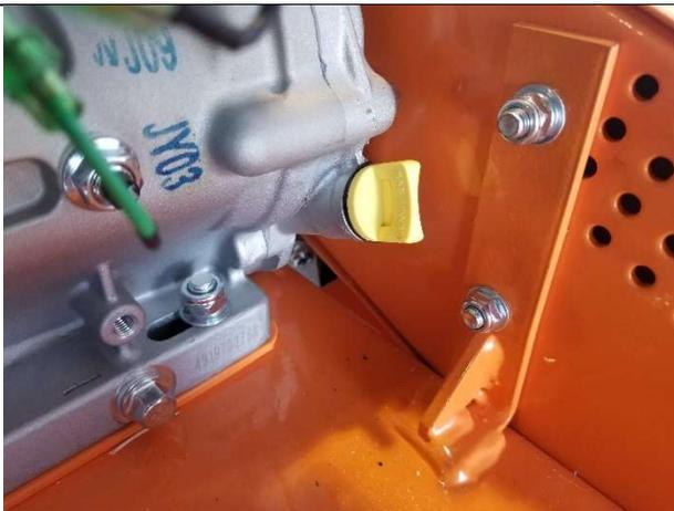
Oil reservoir dip stick. There is one on each side of the engine and they both go into the same reservoir. This is used to fill the engine with oil. Can also be used to check and make sure the correct amount of oil is used. The bolt on the bottom left of the photo is used to drain the oil. Use aluminum foil to direct the oil to a container to keep the unit clean.
