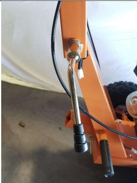
Clamp for adjustable bow handle. Used to loosen the bow handle, make adjustment to bow handle, and tighten to keep secure.
