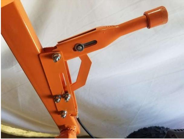
Precision Control Brake for pivot grinding. Stops the left tire from rotating and lets you do wide sweeps across the stumps.
