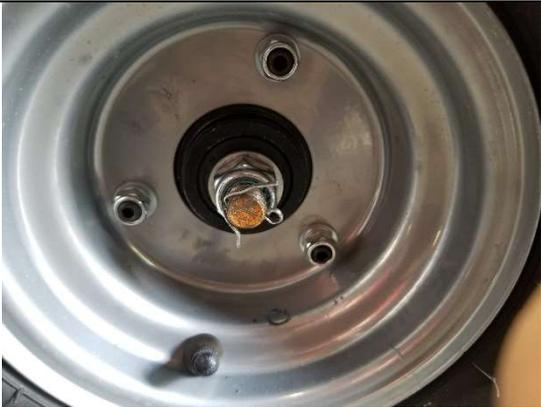
Install washer, nut, and cotter/lock pin.
