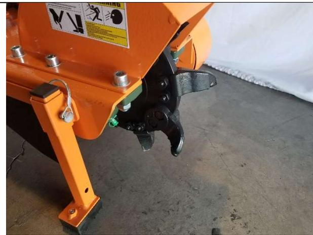
Grinding wheel. Used for grinding the stump.
