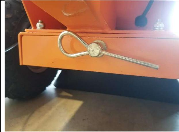
Engine belt adjuster. Used to move the engine forwards and back to tighten or loosen the belt. Loosen the 4 nuts holding the engine to the frame, then make adjustments with this handle.
