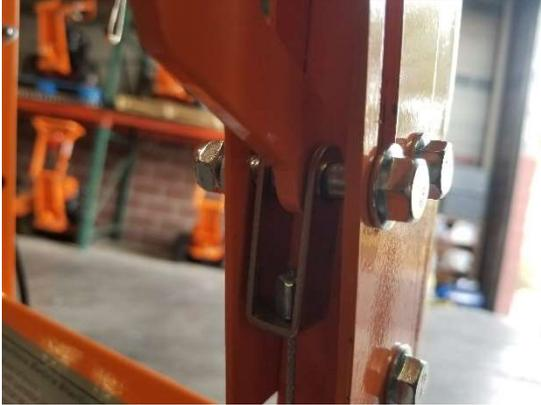
Install bolt, washer, and nut into brake cable/brake arm.
