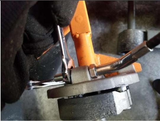
Tighten adjuster and lock nut.
