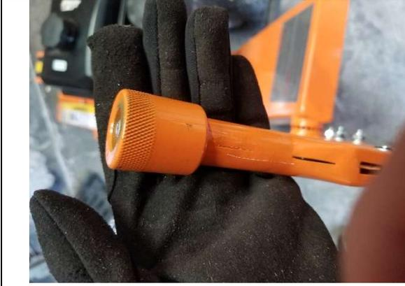
Adjustments to tightness of brake can be made with the adjustable knob. Left to loosen and right to tighten.
